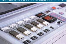
The heating method of barrels is automatic temperature regulating mode, for which each barrel consists of heating/cooling zones, and feed barrel has a cooling zone controlled manually. Water (distilled water) or cooling air is used as a coolant. The panel is build on the body as a desk type.
